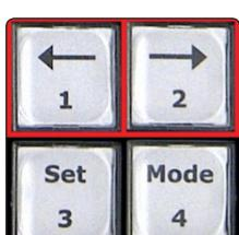
The buttons → and <– can be used to operate the traversing motor
