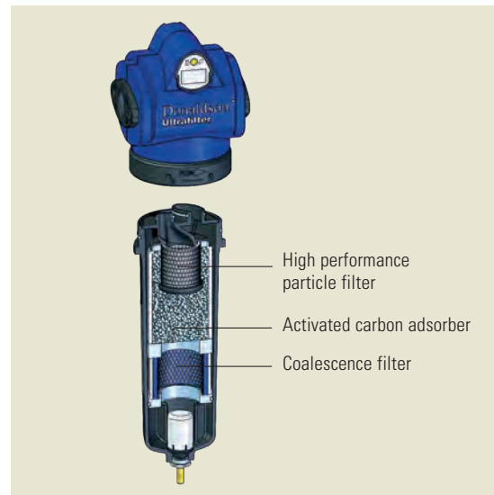
Cross-section of an Ultra-Filter with DF-T element
